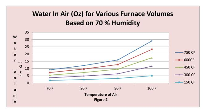
The 300 Cubic Foot curve would be typical of the volume associated with one of our most popular furnaces, the HFL-5748 furnace. We have taken this volume and plotted water volume
